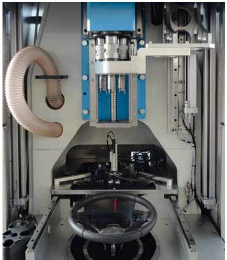
Steering wheel unit (top down) cutting head, moveable measuring system, steering wheel, fixture on top of a hexapod system
