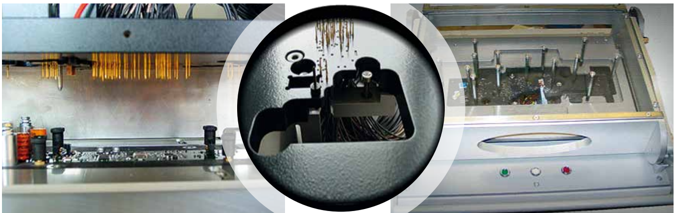
Exchangeable contact unit and VPC interface for multiple test scenarios, left HFT in-line, right laboratory test device for functional test / HFT
