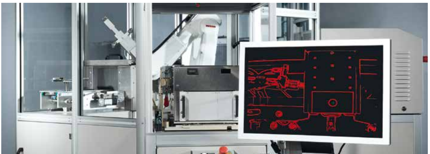
Image pattern recognition of a position marker (right) of a smart camera (center above) for automatic calibration of a robot (center) after changing test setting
