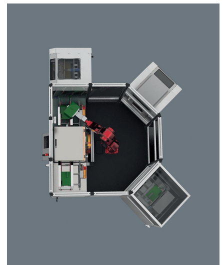
UCMr: UCM demo robot cell with docked UCMi and UCMb for PCB (l. b. & a.) and UCMb for EAS (r. a.) and heating chamber with conveyor (below)
